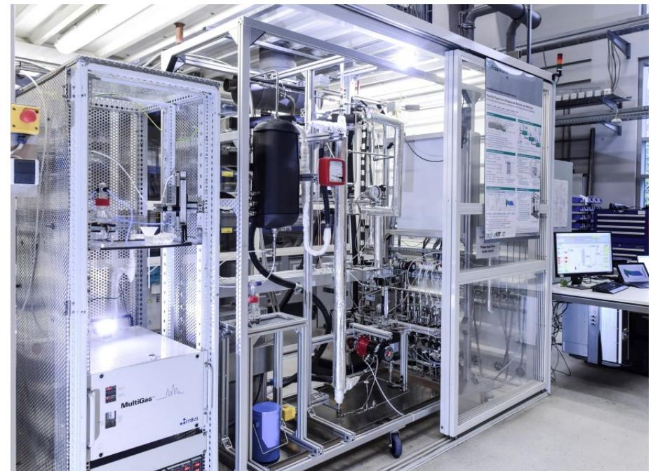
Scale-down test rig for methanol synthesis, 2019
